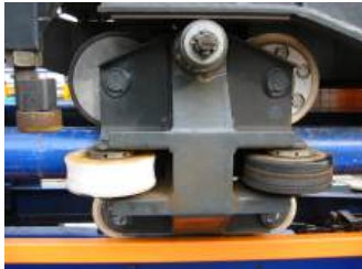
Roller coaster cars have three sets of wheels
