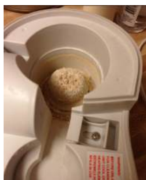
Mineral buildup in a humidifier.
