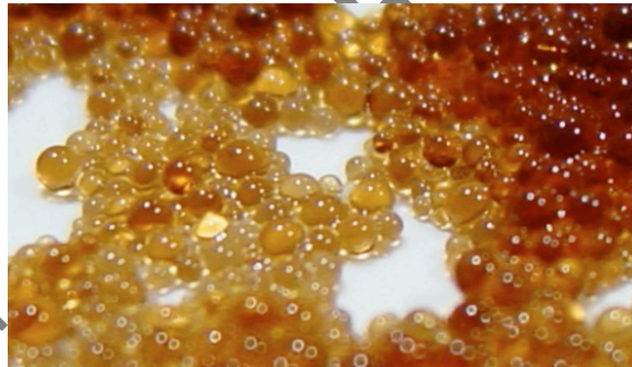
Polystyrene (resin) beads
