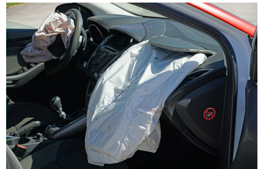
Airbags are inflatable nylon sacks.
