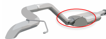
Catalytic converters reduce harmful automobile exhaust emissions.
