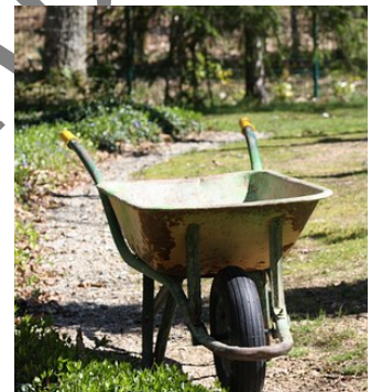
A wheelbarrow is a compound machine.
