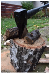
An axe is a type of wedge.
