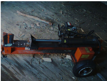
Some log splitters use hydraulics.
